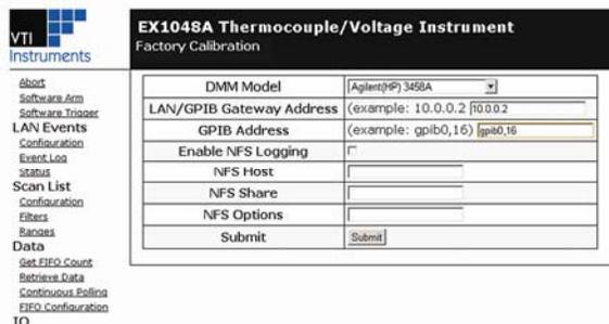
**Figure 4: Embedded Calibration Interface**
