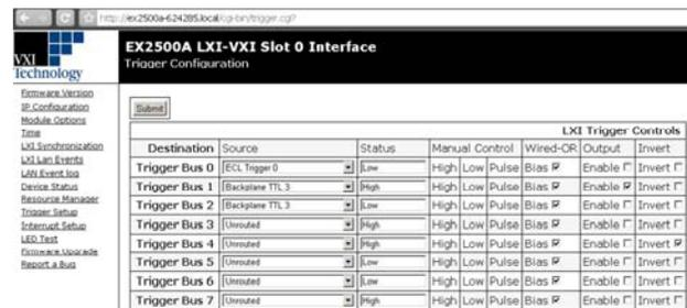
Figure 6: Trigger Bus Configuration
