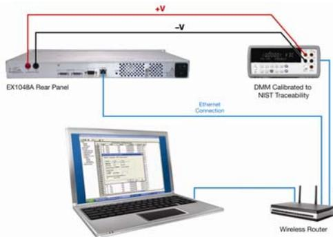
**Figure 3: Embedded Calibration**
