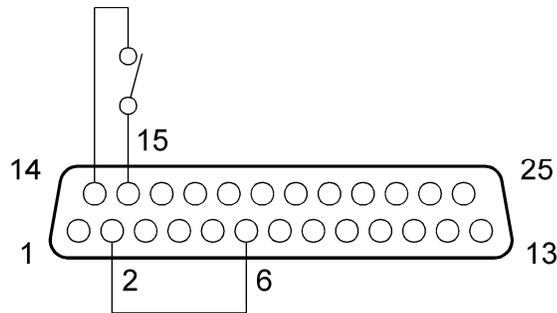
**Figure 4-10. EXTERNAL-OFF with AUXILIARY 5 VDC OUTPUT**
