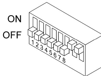
**Figure 4-1. SETUP Switch**
