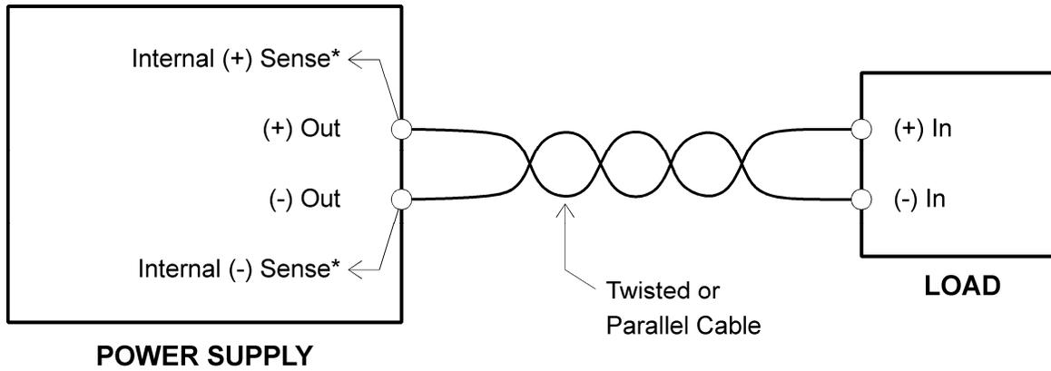
\* SETUP Switch Position-1, REM SNS, Set to OFF
