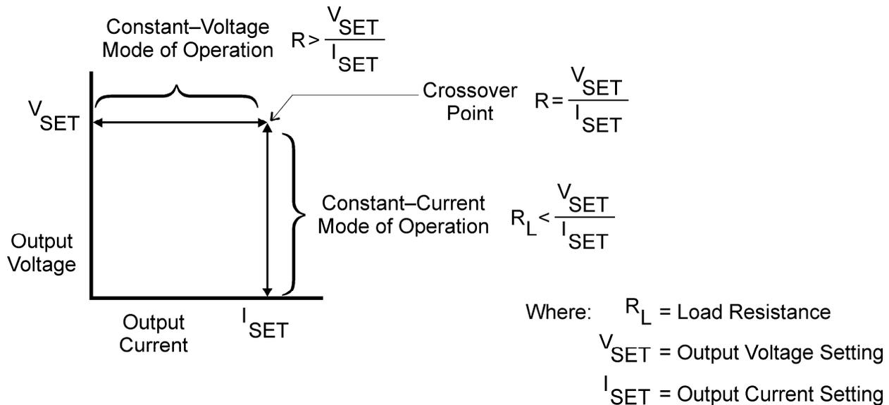
**Figure 3-2. CV and CC Modes of Operation**
