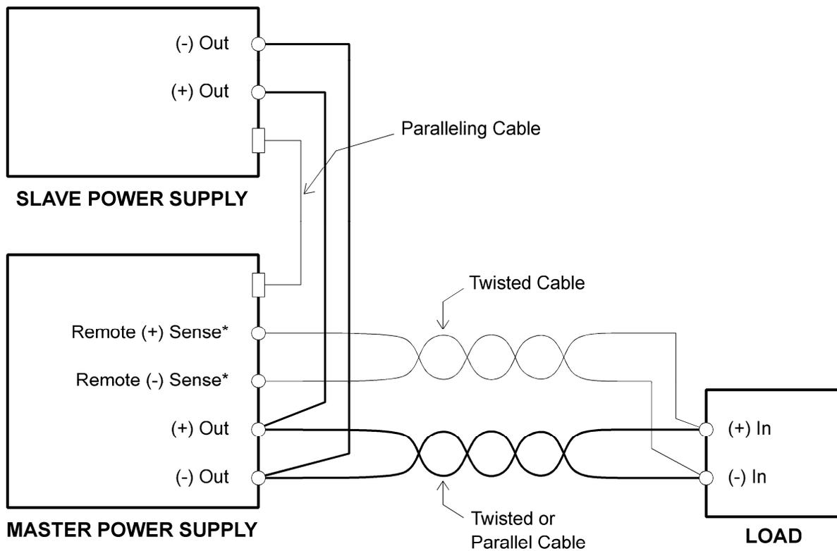
\*SETUP Switch Position-1, REM SNS, Set to ON
