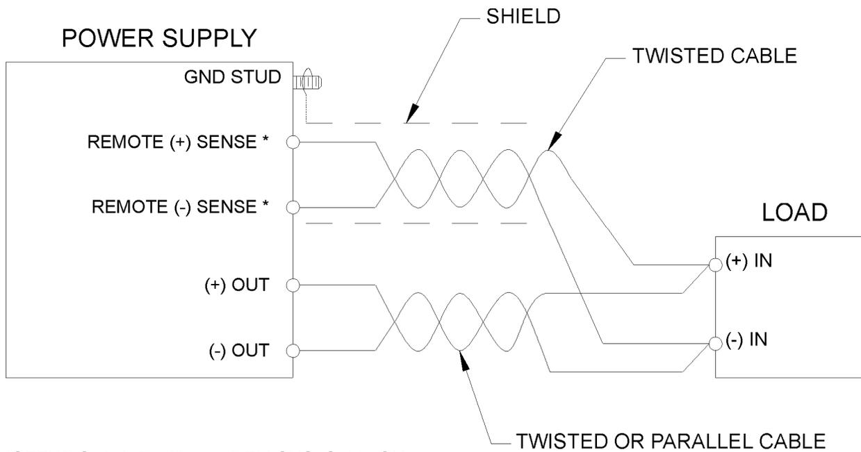
\*SETUP Switch Position-1, REM SNS, Set to ON
