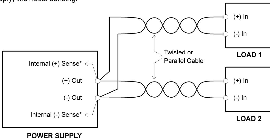
\* SETUP Switch Position-1, REM SNS, Set to OFF
