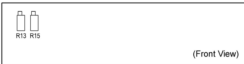
**Figure 5-2. Display PWA Location of Potentiometers**
