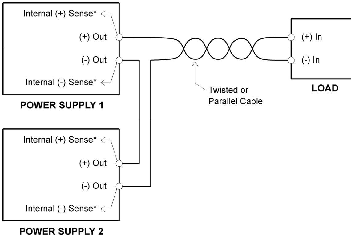
\* SETUP Switch Position-1, REM SNS, Set to OFF
