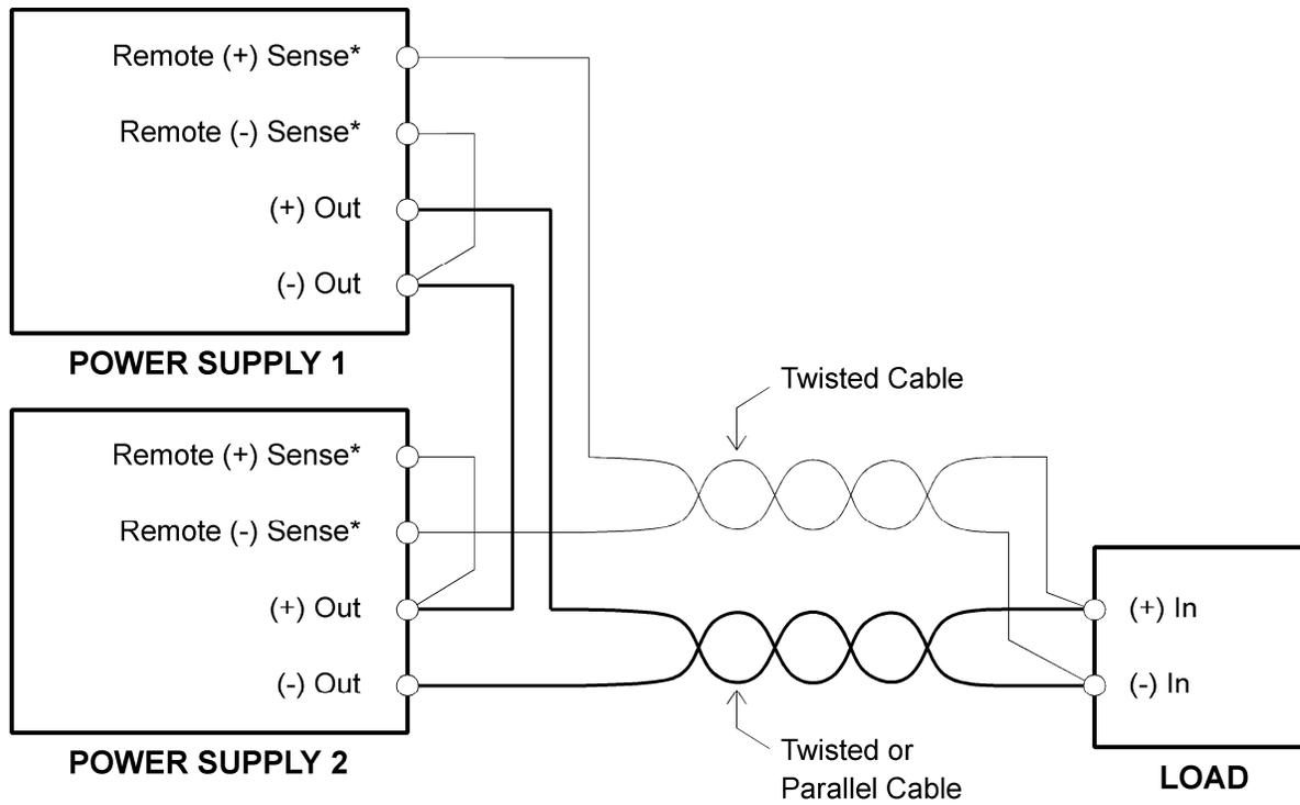
\*SETUP Switch Position-1, REM SNS, Set to ON
