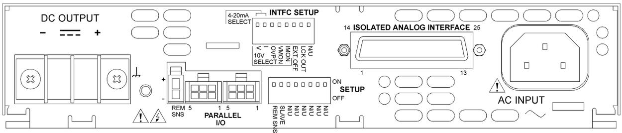
**Figure 2–2. Rear Panel View, High–Voltage Models**
