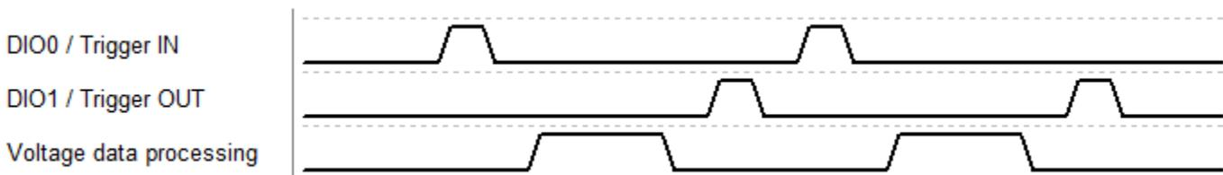
Figure 3: Timing diagram of interface between EX1200 series chassis and external device
