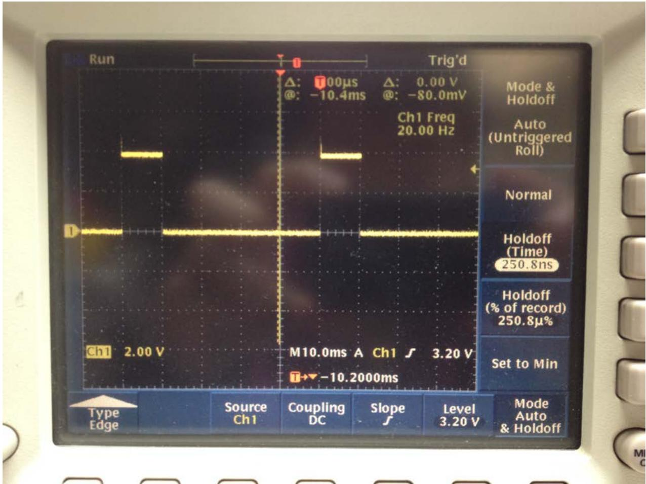
Figure 4: Output pulse (DIO0 / Trigger IN) displayed on scope
