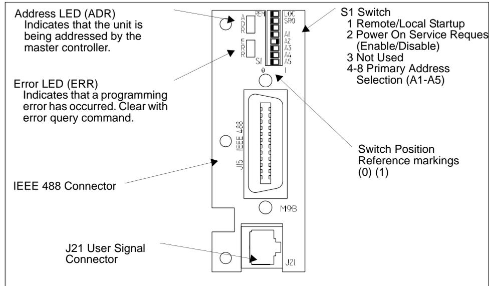
**Figure 2.2** GPIB Interface Subplate
