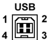
Figure 3-6: USB Connector pin orientation.
