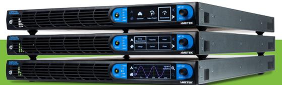
The iX2 technology developed by AMETEK Programmable Power, and incorporated into its California Instruments Asterion AC power sources, allows overcurrent capability up to double its nominal max current resulting in a full 200% overcurrent capability. This allows for full power operation over 75% of the source’s voltage output ranges. This is the widest full power (constant power) on the market today.
